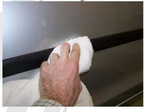
**Step #10** Use a clean towel to apply pressure evenly along the mouldings to secure firmly to vehicle.
