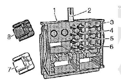
agen AG does not guarantee or accept to the correctness of information in this on the Step 3: Remove locking pin (2) from the radio plug connector (1). Using a pin removal tool from the VAS 1978B, remove the following wires from the radio plug connector and lock them into the
