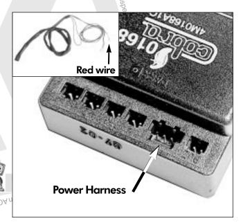
Step#14 Connect the power harness to the **Control Module**
