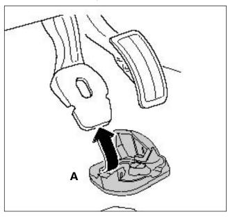
Step#02-Brake pedal cap installation
