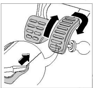
Step#05-Accelerator pedal cap installation
