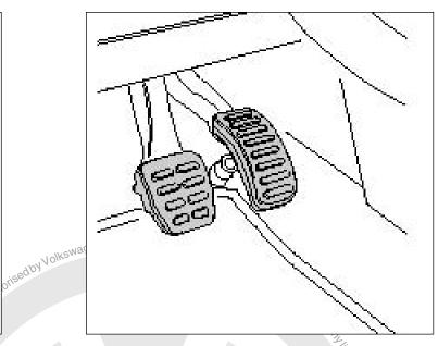
Ensure the pedal caps guides are secured around the accelerator pedal.
