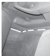
Step#10 Continue to tuck the harness under the sill trim to the bottom of the instrument panel
