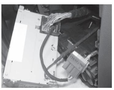
Step#14 Install the blue connector of the adaptor in the Radio Block Connector.
