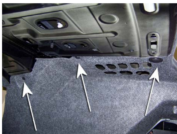
Step #05 Remove the 3 retainer pins located inside the trunk on the under side of the rear deck.
