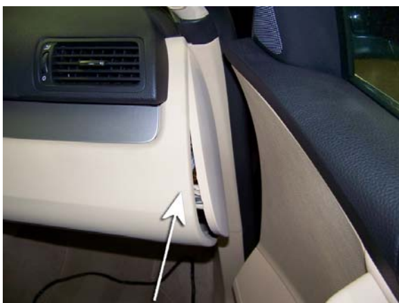
Step #01 Remove instrument panel passenger side end cover
