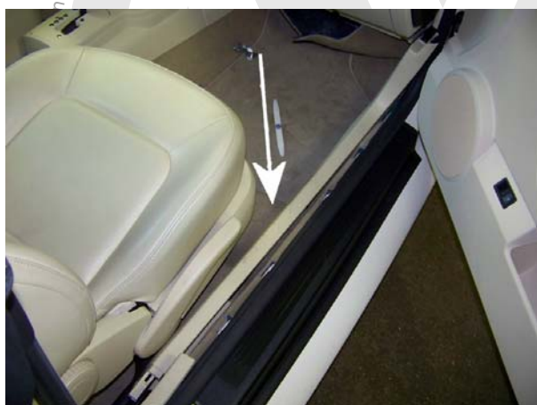
Step #03 Disconnect front and rear sill trim, kick panel and reposition to allow access under carpet
