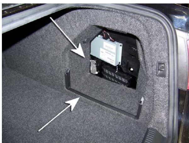
Step #06 Remove the passenger side rear trunk liner panel and tray.
