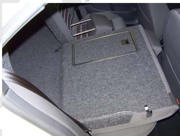
Step #04 Fold down the passenger side rear seat.
