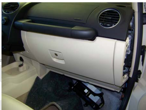
Step #02 Remove the glove compartment (see dash removal)
