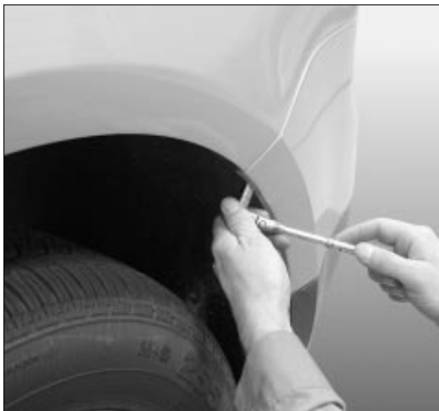
Step#05 Remove rear fascia screws (5/side) from the wheel wells. (T25)
