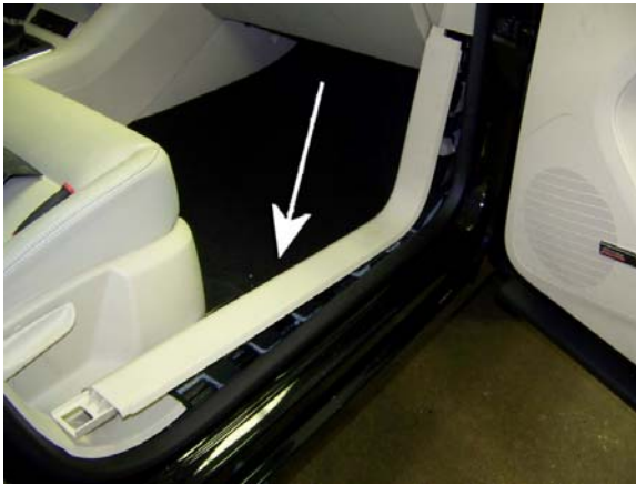
Step #01 Use a trim removal tool to remove the door sill trim.
