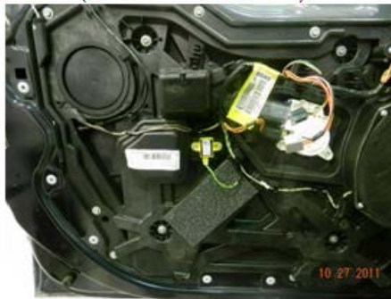
Driver/pass door pressure sensor 7B095557A (CHRY-56054047AC)
