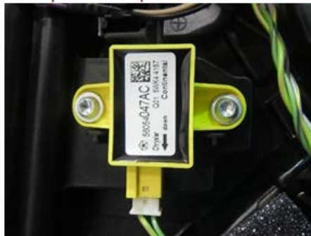
Driver/pass door pressure sensor 7B095557A (CHRY-56054047AC)
