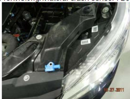
Front left/right lateral crash sensor 7B0909606 (CHRY-56054183AA)
