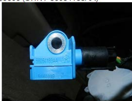
Front left/right lateral crash sensor 7B0909606 (CHRY-56054183AA)
