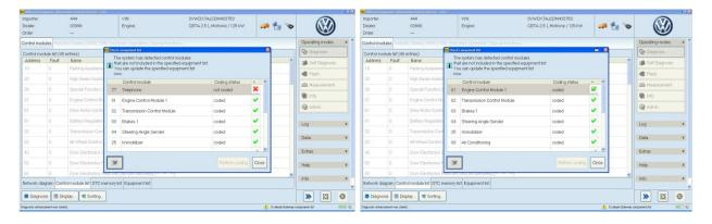
Step 3) The gateway installation list will come up and show the new telephone module is not coded. Change ADW 77 telephone to coded and select perform coding.
