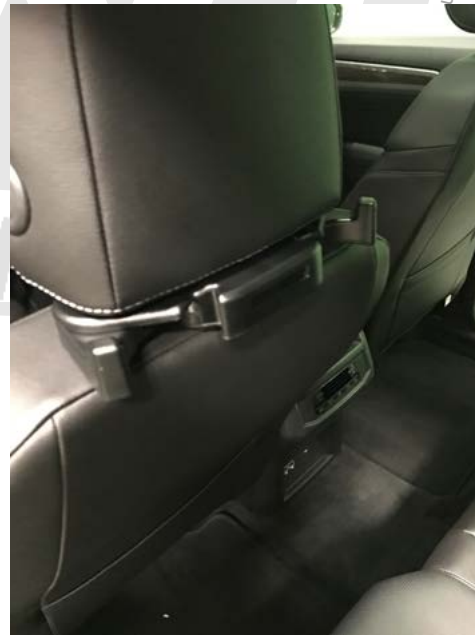
Headrest Bracket with Hooks Extended
