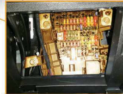
Relay and Fuse Holder SC
