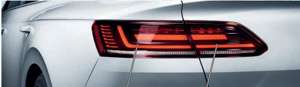
Fixed Section of Tail Light Cluster
