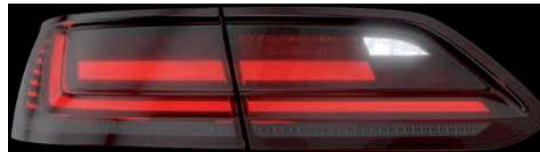
Light Pattern: Tail Light with Reverse Light
